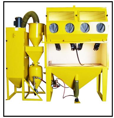
Aboytes Mfg. Cyclone Vortex Reclaiming Systems are designed to keep abrasive media free of contaminants while minimizing media waste.
